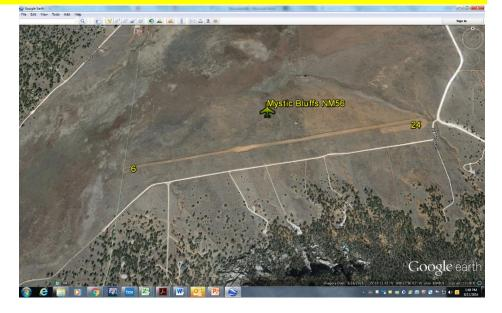
There are power lines right on the threshold of runway 24, plus it slopes significantly downhill. If landing 24 make a right pattern.
