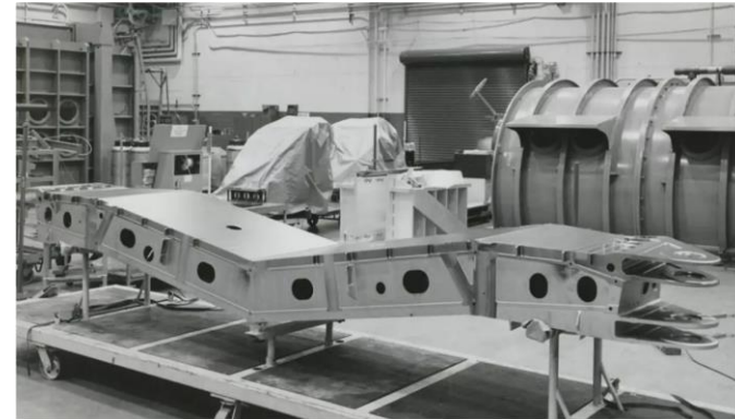
The titanium carry through structure for the F-14 Tomcat was electron beam welded together.
